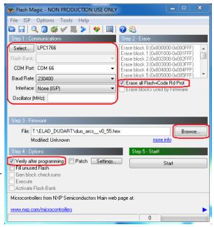
Check the communication with the DUO-ART clicking on "ISP" and then on "Read Device Signature". If the communication with the DUO-ART is working, a new window with some device information is opened.
